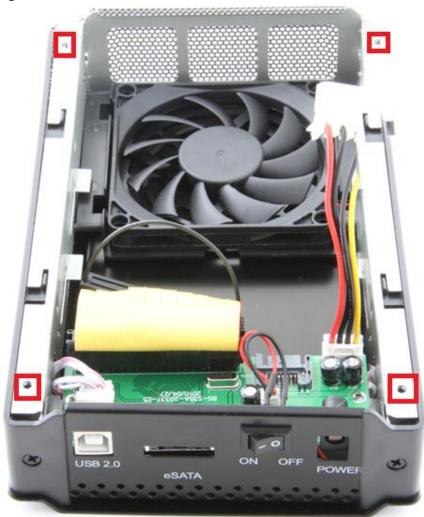
3. Locate the IDE power cable. Connect it to the IDE power port on your drive: Figure A:
